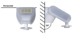
The weather station must be mounted on avertical wall (or a pole) and in the horizontal transverse direction (horizontally).
